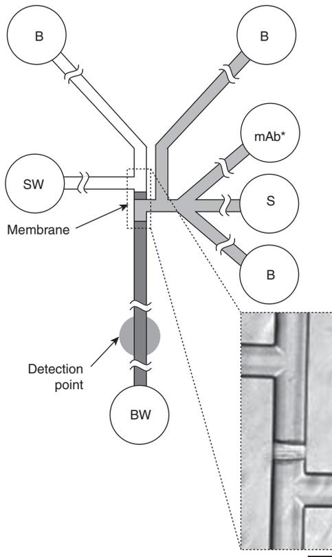
7.11 Microchip electrophoretic immunoassay ( $\mu$ CEI) chip. The device had fluid wells for: S, sample; B, buffer; SW, sample waste; BW, buffer waste; mAb\*, fluorescently labelled monoclonal antibody. The device possessed molecular sieves to enrich the sample and electrophoretically separate the molecular antibody that is bound to an enzyme (Herr *et al.*, 2007).
