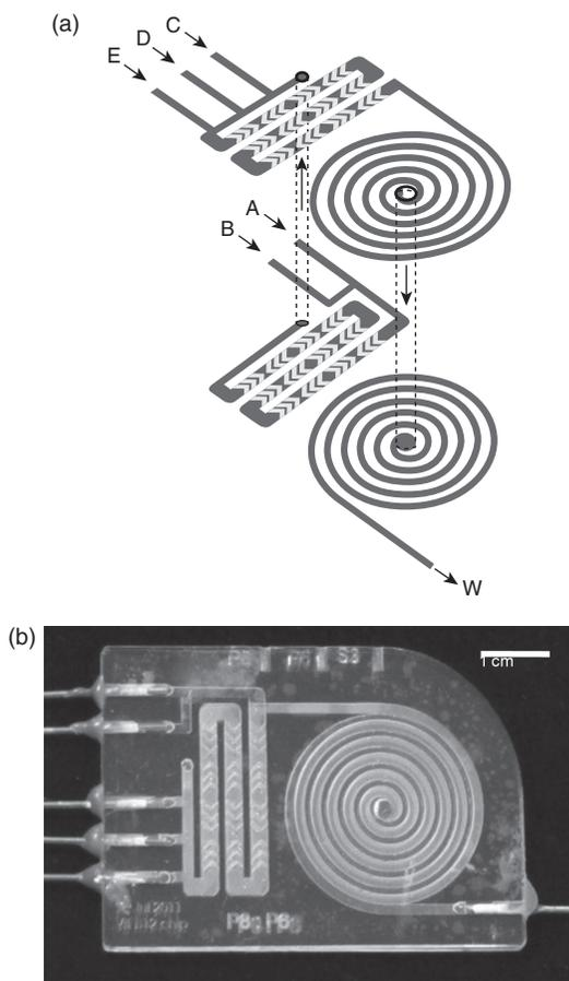
7.9 Microfluidic chip for chemiluminescence based detection of vitamin B<sub>12</sub>. (a) Schematic of the chip with five inlets, two mixing chambers and two spiral detection units, and the fabricated chip (b) (Lok *et al.*, 2012).
