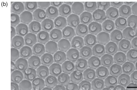
7.6 Microwell arrays for single cell analysis. (a) Fabrication of PDMS-based microwell arrays using polystyrene microbeads, and (b) micrograph image of Ramos cells in each microwell (Scale 20  $\mu\text{m}$ ) (Liu *et al.*, 2010).
